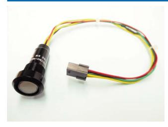
Electro-Mech has introduced its SW44834 switch assembly for DVR Signal Switching. End use application is for operator (bus driver) to actuate switch to time stamp an event on full time DVR safety video recording. During replay, operator can quickly locate event mark on playback to study video more closely. EMC switch features SPST circuitry. bi-color Red/Green illumination for status indication, and wire harness pigtail assembly terminating with a Molex Micro-Fit connector.
