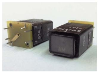
Electro-Mech has introduced its SW44863 splitimage switch series offering an ideal solution for high density instrumentation panels. Typical application is for channel select pushbutton switch in avionics audio control panels. Pushbutton lenses feature hidden legend lenses with multiple LED color options. Typical design includes LED illumination at 5VDC with two independent LED circuits.
